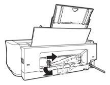
4 Manually rotate the paper feed roller toward you and apply a cotton swab or the like to wipe off dust or stain.
